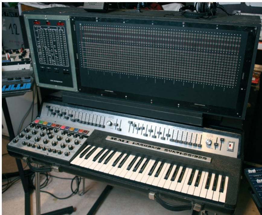
One of the most unusual synths in Jarre's collection is the RMI Harmonic Synthesizer, an early additive synth. On top of it is an even rarer device: the Digisequencer matrix sequencer custom-built by Michel Geiss to Jarre's specification.
